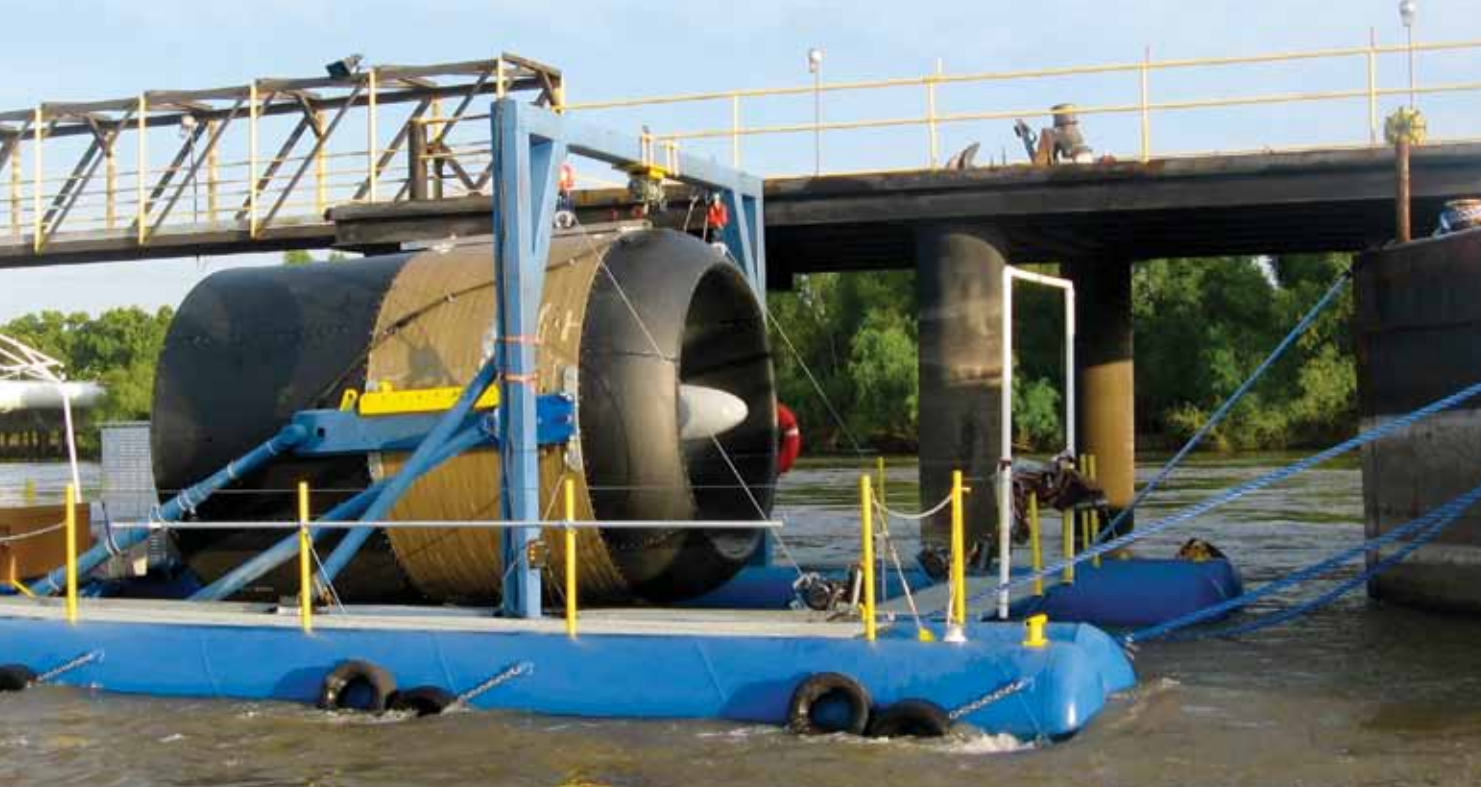
A turbine is deployed in the Mississippi River in Louisiana to capture hydrokinetic energy. Photo courtesy of Free Flow Power
